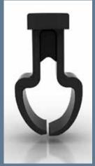
The Magnet clip is the corner stone of the system. The key is the strength with the right flexibility. Fully made of POM, a high performance engineering thermoplastic with excellent dimensional stability even at extreme conditions. Strong yet flexible, low friction coefficient and high abrasion resistance.
